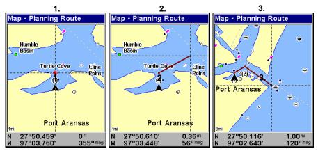
Route creation sequence (left to right): Fig. 1. Set route waypoint (1) at the cove entrance. Fig. 2. Move cursor northeast to set point (2) at channel entrance. Fig. 3. With point (2) set, move cursor southeast to mark channel exit with waypoint (3). In figures 2 and 3, notice the rubber band line extending from the previously set waypoint to the cursor. This line will become the course for the route.
